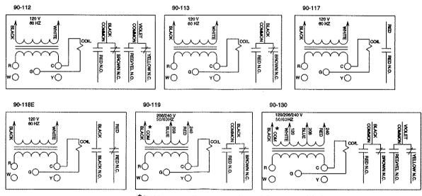
${}^{f *}$  Black is common with respect to transformer winding, not external circuit.
